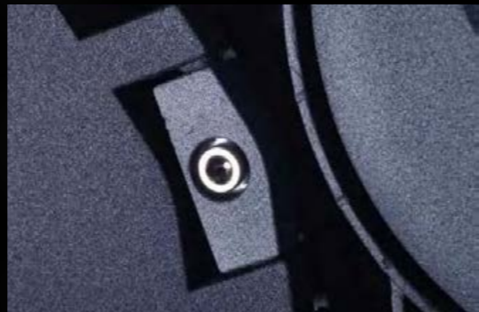
电源腔盖可拆卸 Dismountable power chamber
